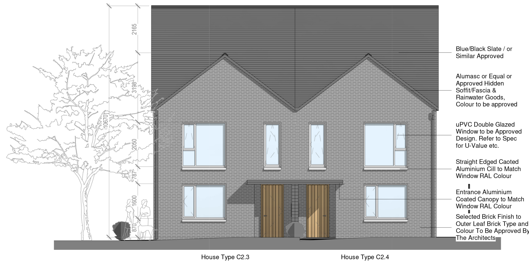
3 Block 7.1 - Front Elevation 1 : 100
